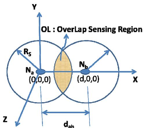
Fig. 1. Over-lapped sensing region of sensor nodes [20].
